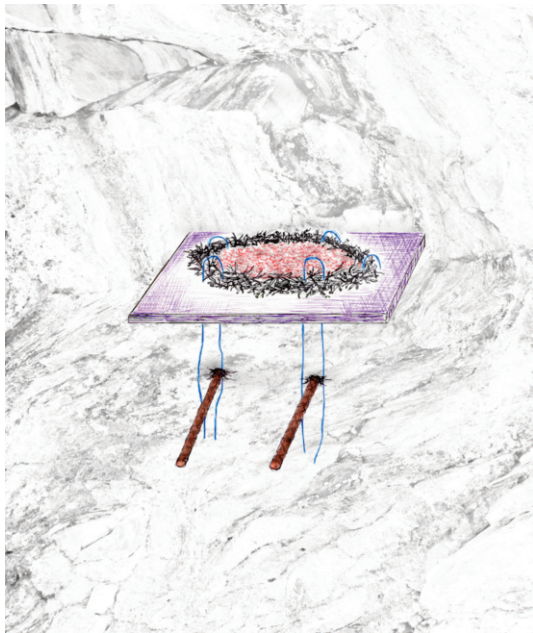
Figure 6. Method of constructing an artificial nest for Gyrfalcons.
